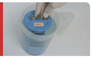
There will be a reaction as the calcium is dissolved. When the reaction ceases (about 10 minutes) rinse the electrode in clean water, wipe the brass terminals dry and check that all calcium has been dissolved. If not, repeat the process with a new solution.
